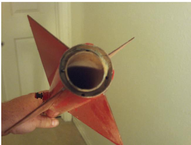
*Thin formica fins, 29mm mount and rail buttons signal a desire for strength and performance.*
